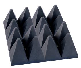
The 3630 series Wide-band hybrid pyramid EM absorber is an 80 mm high absorber that measures 200 mm x 200 mm. It shows good absorption performance in the wide band between 30 MHz and 18 GHz when combined with 6.3 mm thick Ferrite absorber tiles (Part nr. 3600-63). The hybrid pyramid absorber is made out of ferrite and carbon powder and is tuned for perfect performance over Ferrite absorber tiles.
