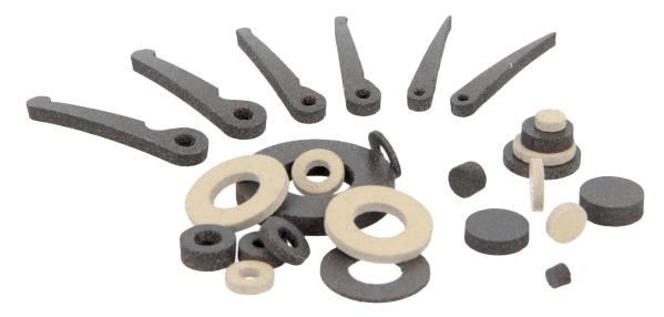
Standard Nickel-graphite conductive rubber is used for EMI applications. The rubber is made conductive by incorporating small conductive metal particles throughout the material. It can provide an EMI-proof and watertight seal in narrow constructions. But they are also useful for EMP protection, wave-guide applications and against static electricity.
