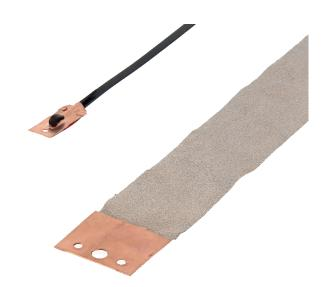
Stretch materials up to 30% without permanently deforming. On both sides copper clips for mounting the sensor on the product with little resistance loss. Precise movement measuring by changing resistance in the material. Two types of material; conductive fabric and conductive rubber. Length of the sensor can be specified on request. The sensor doesn't have any sharp edges so it can be used on skin.
