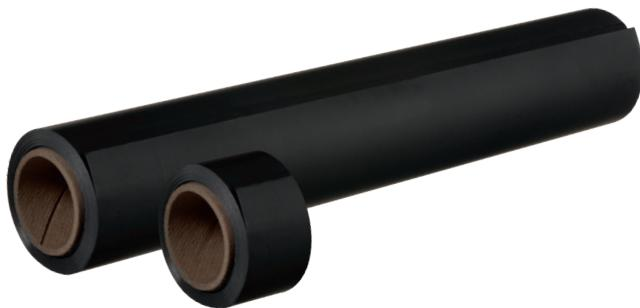
Semi-Conducting non woven tapes primary function is to equalize the field current around the conductor or core and to ensure electrical contact with the earthing system. This reduces the electrical stress on the insulation material and enhances performance. They can also be used to prevent electrolytic corrosion of metallic armour layers.
