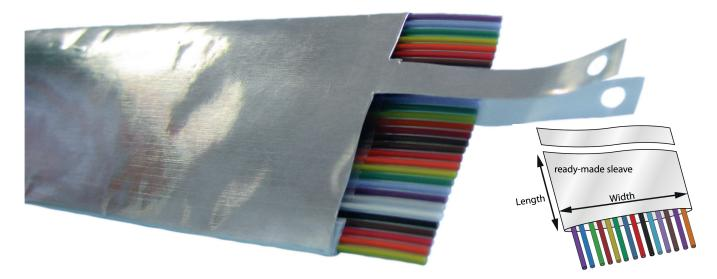
The ready-made sleeve (EMI-screening sleeve) for flat cables allows easy cable routing during assembly. The material is a highly conductive Amucor film offering full 360° protection against electromagnetic radiation. Shielding performance can even be improved using optional grounding connections.
