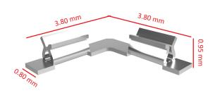
This clip is to be mounted onto the surface of a PCB (SMT) and offers a fast solution for assembling RFI/EMI-shielding cans to PCB's. This clip eliminates the need for through holes and post reflow operations on the PCB. For best performance, the shielding clip should be mounted on the PCB ground pattern. This can be done by hand or by vacuum pick-up nozzle (automated).
