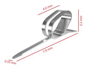
This clip is to be mounted onto the surface of a PCB (SMT) and offers a fast solution for assembling RFI/EMI-shielding cans to PCB's. This clip eliminates the need for through holes and post re-flow operations on the PCB. For best performance, the shielding clip should be mounted on the PCB ground pattern. This can be done by hand or by vacuum pick-up nozzle (automated).
