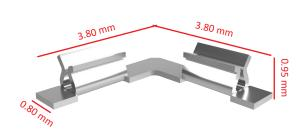
This clip is to be mounted onto the surface of a PCB (SMT) and offers a fast solution for assembling RFI/EMI-shielding cans to PCB's. This clip eliminates the need for through holes and post reflow operations on the PCB. For best performance, the shielding clip should be mounted on the PCB ground pattern. This can be done by hand or by vacuum pick-up nozzle (automated).
