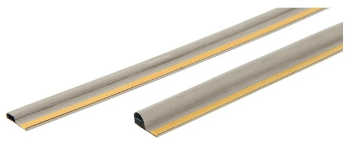
7200 series P-shape EMI shielding gaskets consists of a P-shaped closed cell foam core which is covered with a conductive fabric with a copper-nickel metal coating (material code T) or highly conductive Amucor foil (material code A).
