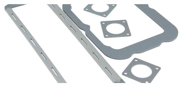
Oriented wire shield 5711-5722 is a composite gasket material consisting of a large number of small wires embedded and bonded in solid or sponge silicone, or fluorosilicone elastomer for oil resistance.
