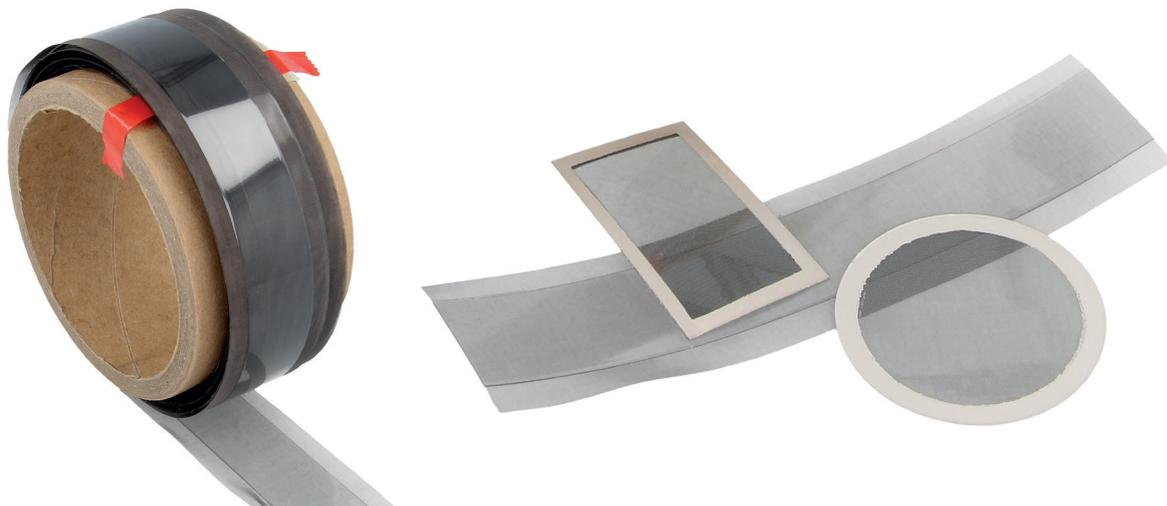
Mesh foil is a very fine, electrically conductive wire mesh laminated between two layers of scratch-resistant transparent foil. The wires are so fine that they can hardly be seen with the naked eye. The product is very strong but it still bends easily. It is easy to apply Mesh foil onto glass, acrylic and polycarbonate, either by hand or with a laminator. It can be supplied with or without self-adhesive.
