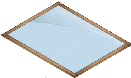
(C) With copper edges for grounding
