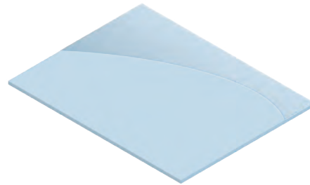
(N) Without a special contact edge; there still is electrical conduction at the coated side of the glass.
