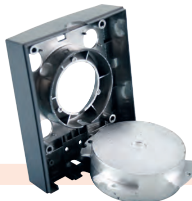
Figure 78: Example of plastic housings with shielding paint.
