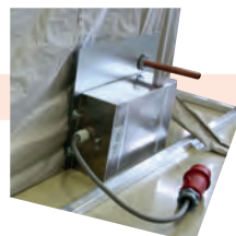
Wave guide & power line filter
