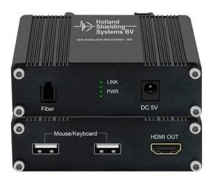
HDMI 4K 60Hz Over Fiber Extender, consists of a Transmitter and a Receiver unit that allows you to extend HDMI 2.0 and USB HID signals up to 300 meters over LC OM4 MM Fiber Optic Cabling. The HDMI KVM extender delivers up to 4K 60Hz UHD picture quality to your remote display with support for 4:4:4 chroma sampling.
