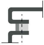
1. Endless gasket used in a flat lid on a curved housing construction
