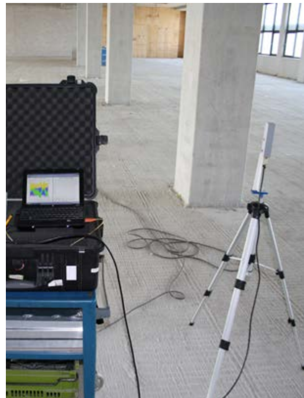
Measuring radiation in adjacent room
