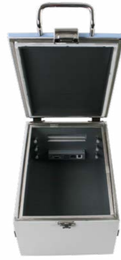
Medium shielded box to block wireless communication during testing and measurements
