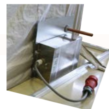
Wave guide & power line filter
