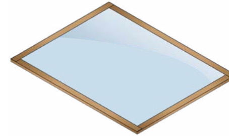
(C) With copper edges for grounding
