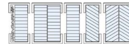
Figure 81: From left to right, Honeycomb with dust filter, cross cell, single cell straight, single cell slant 45 degrees, double slant to prevent eavesdropping
