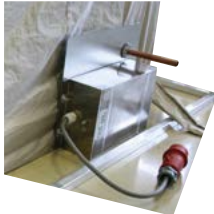
Wave guide & power line filter
