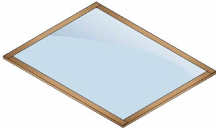
(C) With copper edges for grounding
