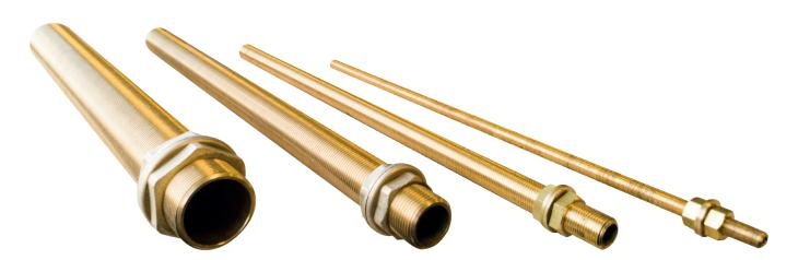
Waveguides are specially designed metal tubes in order to block electromagnetic waves. They are available in almost any size depending on frequency. Attenuation curve is in relationship with diameter. Any non metallic material can be fed through the waveguide such as optical fiber, water, gas or air.
