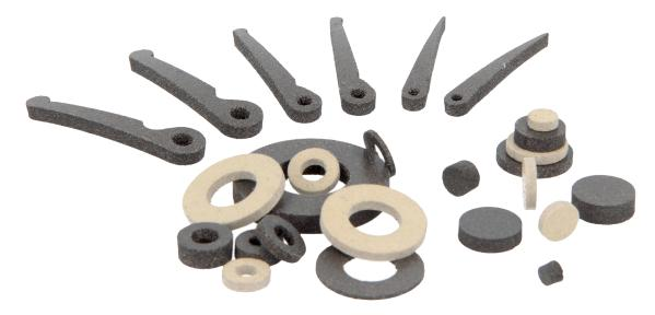
Standard Nickel-graphite conductive rubber are used for EMI applications. The rubber is made conductive by incorporating small conductive metal particles throughout the material. It can provide an EMI-proof and watertight seal in narrow constructions. But they are also useful for EMP protection, wave-guide applications and against static electricity.
