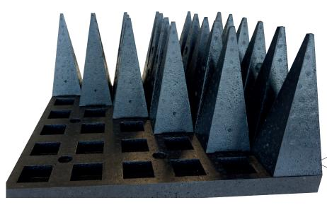
The Polypropylene (pp) based microwave( electromagnetic wave) absorber is looking the same as our Polypropylene (pp) based hybrid pyramid absorber 3700 but this absorber is used on the high frequeny range. The absorber is designed for antenna measurement in anechoic rooms and solution for Antenna Pattern Measurement (APM), Antenna Test Range (ATR), Radar Cross Section (RCS) and Electronic Warfare Test (EWT) chambers.
