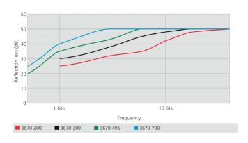
**Please note:** For the data below 500MHz, it is obtained by low-frequency coaxial test method (GJB5239-2004); while for the data above 1GHz, it is obtained by far-field RCS test method (GJB2038A-2011) The performance data listed in the above table is the guaranteed data, and the measured data would be equal to or better than the guaranteed data. Certification: CE ROHS
