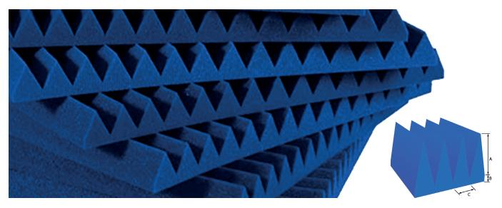
PU foam based wedge absorbers has the properties similar to the pyramid absorbers with same height, it also has excellent performance in 100MHz-110GHz. It is mainly applied in large compact anechoic chamber and tapered anechoic chambers, the main advantage is to reduce the back scattering of pyramid absorbers and obtain higher quietness of quiet zone.
