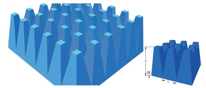
The 3660 series PU foam based Hybrid absorbers product is similar to our standard pyramid absorbers, but having the tips of the pyramids truncated. This saves space in small chambers and provides a more rugged product, eliminating the possibility of tip breakage.
