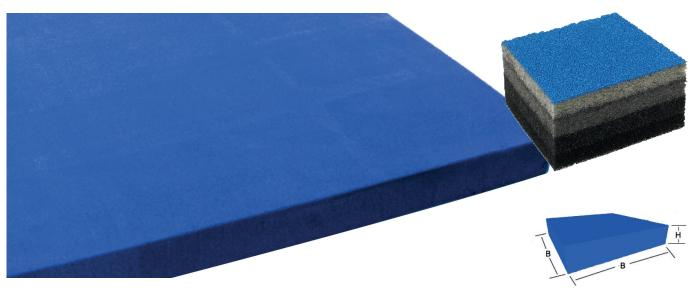
These absorbers can be used at higher frequencies than traditional shielding and can also be used with other EMI/RFI shields to extend frequency range. The microwave absorbers can be installed easily with (PSA) pressure sensitive adhesive, often directly onto high-frequency board-level components to absorb unwanted radiated and surface wave EMI/RFI and meet FCC requirements without shielding.
