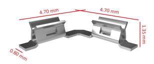
This clip is to be mounted onto the surface of a PCB (SMT) and offers a fast solution for assembling RFI/EMI-shielding cans to PCB's. This clip eliminates the need for through holes and post re-flow operations on the PCB. For best performance, the shielding clip should be mounted on the PCB ground pattern. This can be done by hand or by vacuum pick-up nozzle (automated).
