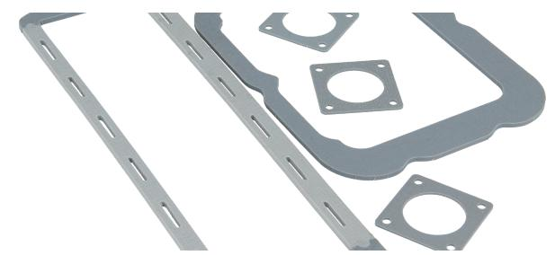
Oriented wire shield 5711-5722 is a composite gasket material consisting of a large number of small wires embedded and bonded in solid or sponge silicone, or fluorosilicone elastomer for oil resistance.
