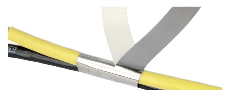
Mu-ferro foil/tape is a thin foil; its thickness is only 0.023mm. It combines excellent soft magnetic properties with unusual mechanical hardness and flexibility. This means that tight bends can be realized with only very slight impairment of permeability. The fine strip thickness and comparatively low electrical conductivity permit effective shielding even of higher-frequency fields.
