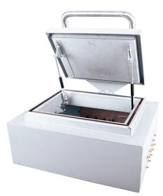
This EMI/RFI-shielded box has up to 120dB reduction of RF signals up to 5 GHz. This makes the shielded box ideal for testing cellular handsets, RFID, Bluetooth, Zigbee, WiMax, WLAN or similar wireless devices. The box can be constructed in any size required.
