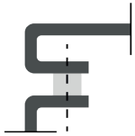
1. Frame gasket used in a flat lid on a curved housing construction
