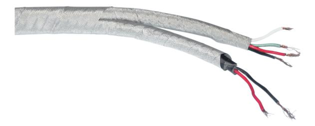
Flexible cable shield is suitable for EMI-shielding applications where flexibility is required, for example when cables have small diameters. The material guarantees superb EMI shielding performance. The product is supplied on rolls and can be wrapped around the cables. Flexible cable shield is available in **Amucor** or in **conductive fabric**, with or without (conductive) self-adhesive.
