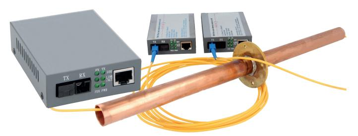
Our 7894- Fiber-optic ethernet converter set offers a shield-ed-room feedthrough for high-speed Ethernet/UTP communication links. The fiber-optic ethernet converter set is used to convert a 10/100/1000 Base-T signal to a 10/100/1000 optical signal, so you can use your internet connection or for example your videocamera connection inside or outside the Faraday cage while maintaining over 140 dB of room attenuation.
