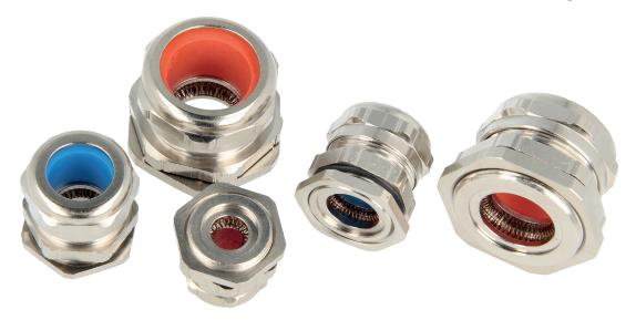
The Cable Entry Gland provides an excellent EMP/RFI shield for screened cable which pass through enclosure walls. A round or threaded hole is required to mount the gland. (The gland can also be welded or soldered into the enclosure wall).
