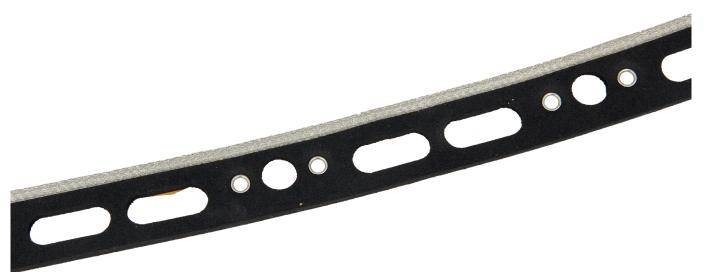
This gasket is used for screwed connections for EMI and EMP protection. The water seal is made out of flame retardant neoprene foam. In the water seal are not only holes for bolts but also holes to make the foam more easy to compress. This makes it so that it can be used to screw thinner plates together without bending.
