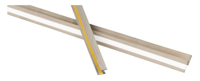
A CNC extrusion system has been developed to manufacture EMI shielding gaskets in a wide range of shapes and dimensions. Thanks to this system there are no additional tooling costs, which makes it interesting for smaller quantities or special constructions. The metal-cladded, flame-retardant gasket can be manufactured in several rigidities and is very compatible with aluminum, zinc-plated steel, AluZinc, stainless steel, copper, etc.
