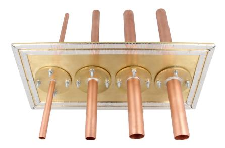
Waveguides are specially designed metal tubes in order to block electromagnetic waves. They are available in almost any size depending on frequency. Attenuation curve is in relationship with diameter. Any non metallic material can be fed through the waveguide such as optical fiber, water, gas or air.
