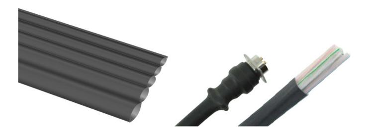
The Conductive shrinking sleeves are used for cable and connector terminals to provide efficient EMI shielding. The sleeve is a combination of heat shrink polyolefin tube and a flexible conductive layer that can shrink. When the sleeves are heated the conductive layer will shrink at the same time.
