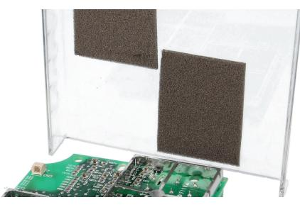
Compartment shield foam is a highly conductive foil laminated with a high-deflection, low closure-force foam layer. The housing itself is used to close the separations on the PCB. The high-deflection, low closure-force foam is also available combined with conductive fabrics or non-wovens.
