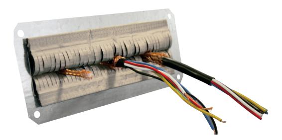
A shielded cable-entry system to mount, ground and shield several cables or bundles of cables simultaneously. The highly conductive, flexible EMC gasket between which the cables are entered into the enclosure guarantees excellent shielding performance between 1 MHz and 10 Ghz. Standard material for the plate is galvanized steel.
