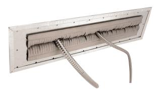
We can deliver cable-entry shield as a turnkey implementation- we call this the Entryshield instant version 4915. This instant version is a Mu-ferro plate of 2 mm thick with the entry shield already mounted in this plate. The instant version is like a letterbox flap, only for entering EMI/RFI-shielded cables. This version is easy to fit into a EMI/RFI-shielded box, EMI/RFI-shielded room or Faraday cage.
