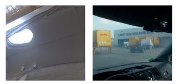
Mounting the shield for signal-jammer cars is achieved easily, by means of suction cups to the windows. The shield we supply will be customized for your make and model car.
