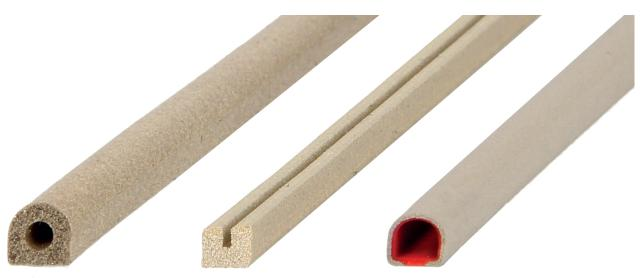
The rubber in these profiles is made conductive by means of small conductive metal particles, distributed throughout the rubber. It can provide an EMI-proof and a pressure watertight seal in narrow constructions.
