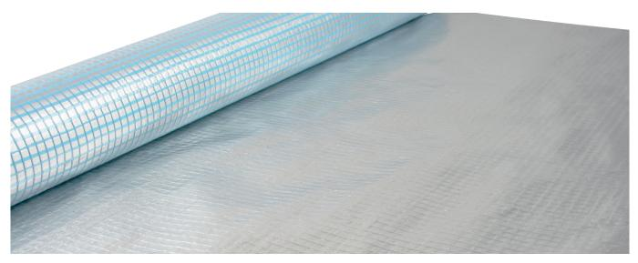
Many EMI problems can be solved easily by the use of Amucor foil or tape. When there is a very broad and strong shielding foil required, than our 4706 Amucor foil with reinforcement net can provide the solution. The shielding foil can be produced with or without (conductive) self-adhesive and an optional insulation layer.
